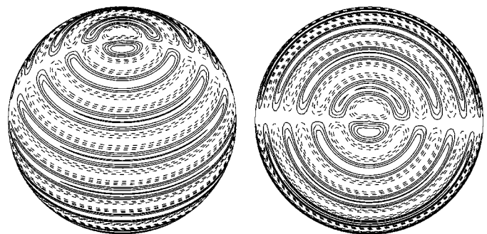
FIG. 7. Contours of radial flow u_r at the middle surface of the spherical shell for Pr=7.0 with the initial condition \Psi(q=0, l=18, m=1) . On the left panel, we view it from 45^\circ from the north pole while the right panel is viewed from the south pole.
